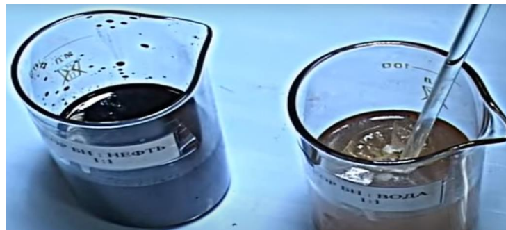
Figure 22. AKOR-BN material: Result of reaction with oil and water
